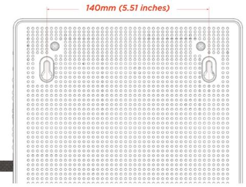
**Note:** The screws should protrude from the wall so you can fit the device between the head of the screws and the wall. If you install the screws in drywall, use hollow wall anchors to ensure the unit does not pull away from the wall due to prolonged strain from the cable and power connectors.
