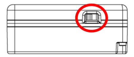
The power switch is highlighted in red. The switch is shown in the Off position. Slide it towards the USB-C port to turn power On.
