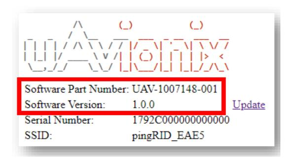
Annually, or as required, confirm the displayed "Software Part Number" and "Software Version" are current per Service Bulletins listed at: <a href="https://uavionix.com/support/pingrid/">https://uavionix.com/support/pingrid/</a>
