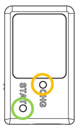
The charge LED is highlighted in orange. It will illuminate in orange while charging and extinguish when charging is complete.
