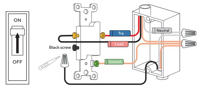
3. Turn off the circuit breaker and label the Line wire.
