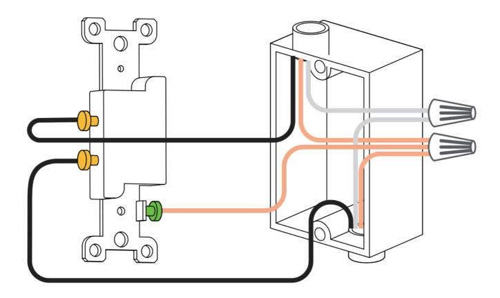
**WARNING:** Neutral wire is required to install the smart switch. If you can't find the neutral wire, please call an electrician for help.
