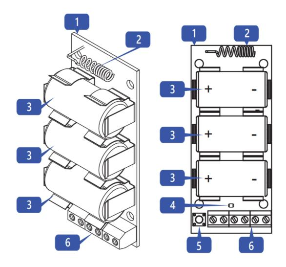
**U-Prox Wireport** – is a wireless module with 3 inputs, designed to connect wired equipment (detectors, IR barriers etc.) to wireless U-Prox control panel. It has 3V controlled power output and can be built into detectors. The device is connected to the control panel and is configured with the U-Prox Installer mobile application.
