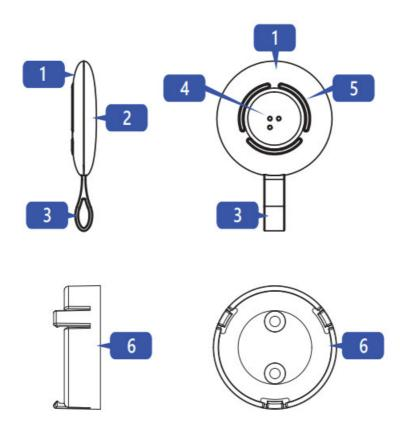
U-Prox Button – is a wireless key fob / button designed to control the U-Prox security system.
