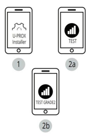
Due to Grade 2 requirement RF link works with reduction of power in 8 dB
