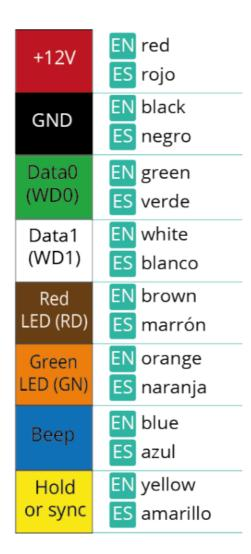
We recommended to use following whiring when reader connected to the control panel with twisted pair.
