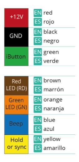
We recommended to use following whiring when reader connected to the control panel with twisted pair.
