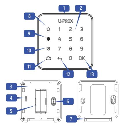
U-Prox Keypad G1 – is a wireless keypad designed for arming and disarming, displaying alarms and device status, as well as interaction with the user of the alarm system.
