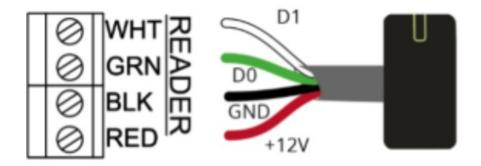
The current consumption of each external reader connected to the +12V terminal must not exceed 100 mA. If long-range readers draw more than 100 mA, their supply voltage must be provided from a separate source.
