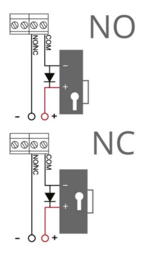
When using the relay contacts to control an inductive load (e.g., an electromagnetic lock), a flyback diode should be installed in reverse across the coil power supply to avoid contact damage.
