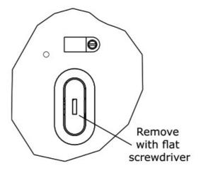
5. Thread water line through back panel hole (with bushing).
