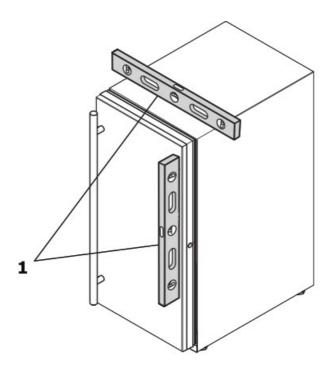
2. If the unit is not level, adjust the legs on the corners of the unit as necessary.
