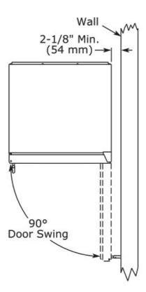
Units have a zero clearance for the door to open 90°, when installed adjacent to cabinets. Stainless Steel models require 2-1/8" (54 mm) door clearance to accommodate the handle if installed next to a wall.
