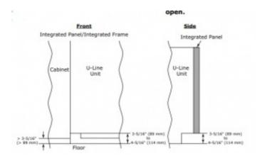
\* Panel can extend beyond the door frame. \*\* A minimum of 1" (25 mm) from the flooris required for proper ventilation.
