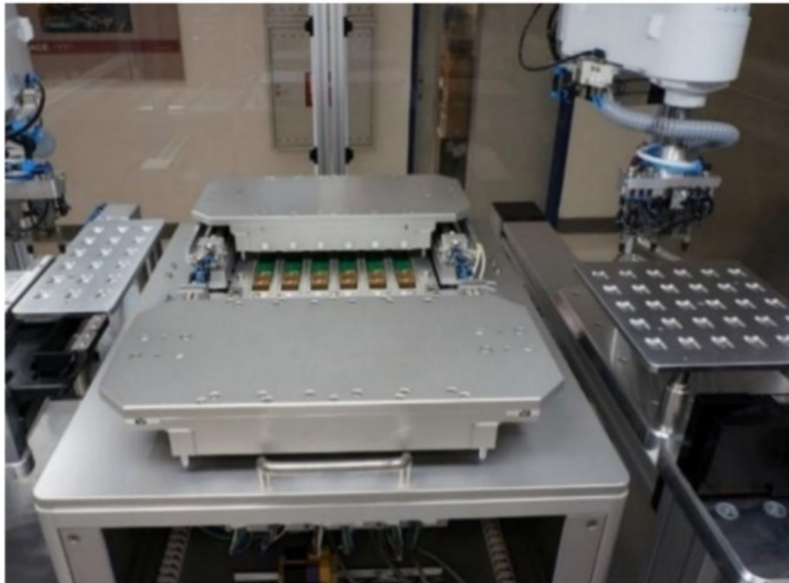
Figure 14: Automatic test equipment for module test
