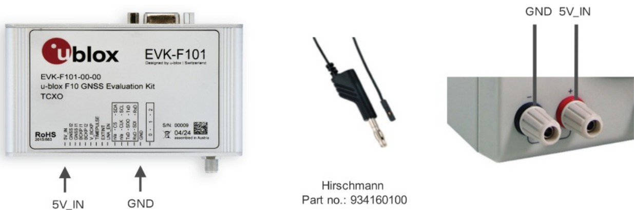
Figure 3: EVK-F101 5.0 V DC power supply example
