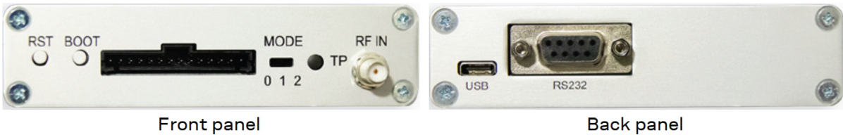
Figure 2: The front and back of EVK-F101
