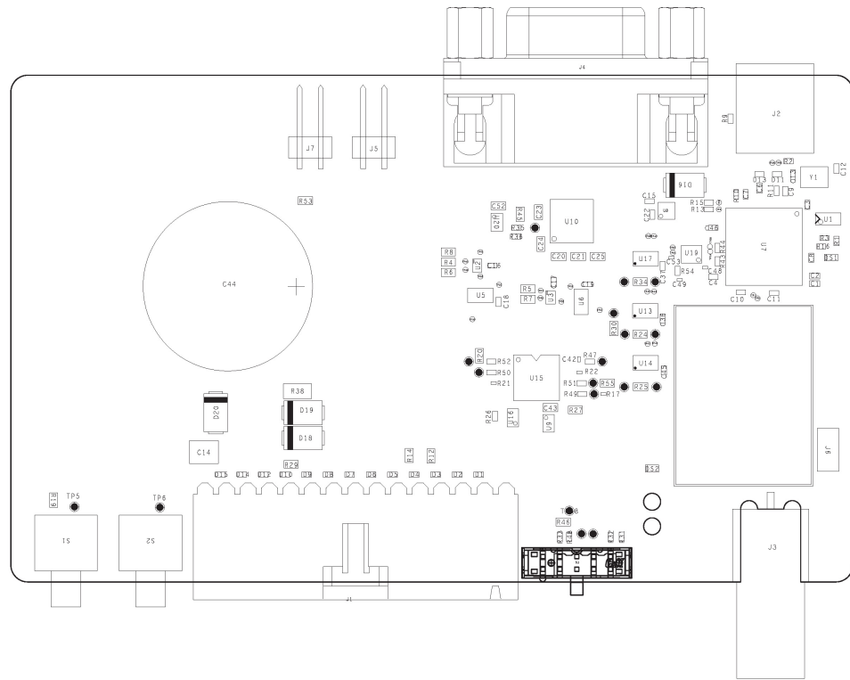
Figure 7: EVK-F101 board layout
