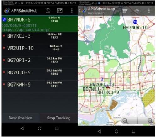
After the setting is completed, enable: start Tracking. At this time, the red indicator light inside the Bluetooth converter box is long, indicating that the APRSDROID is connected to the Bluetooth converter box. When the FT400 receives the decoded beacon, it will immediately transmit to the APRSDROID via Bluetooth. To the APRS list, you can also see the specific location or trajectory of the other party through the APRS map in real time.
