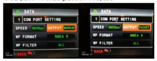
\*Select waypoint, the beacon output has a call sign and GPS coordinates \*Select : packet, the beacon output has call sign, GPS coordinates and beacon text
