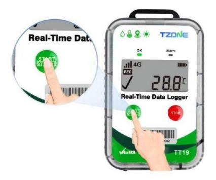
7. Step7: Install the device at the temperature monitoring site and send the data,if the signal grid " is displayed in the upper left corner of the device, it means that the machine has successfully sent data.
