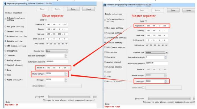
**Step 3:** Configure the IP connection work timeslot same with the master repeater.
