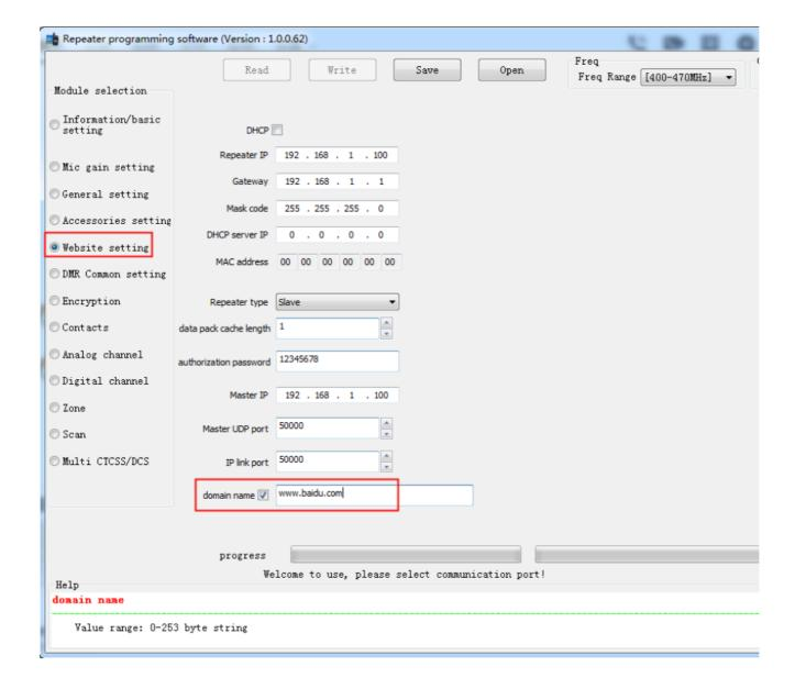
In the above configuration, the WAN side UDP port and the master repeater use the same UDP port. If the WAN side UDP port is not same with the master repeater UDP port, the master UDP port of all Slaves must be modified as the WAN side UDP port.
