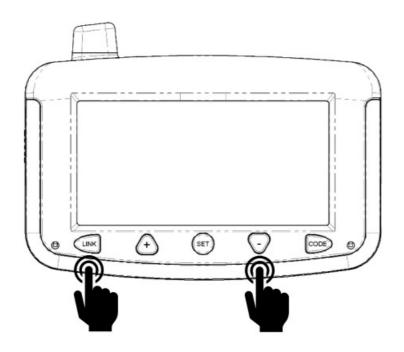
PRESS THE "LINK" AND "-" BUTTON SIMULTANEOUSLY THE CARAVAN / TRAILER ICON IS REMOVED FROM THE SCREEN
