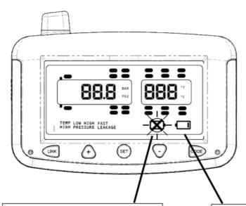
THIS ICON FLASHES WHEN THE SENSOR BATTERY VOLTAGE IS LOW.
