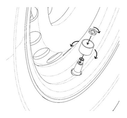
NOTE: WHEN THE DUST SHIELD IS FITTED FOLD IT BACK ON ITSELF. THIS MAKES IT EASIER TO FIT
