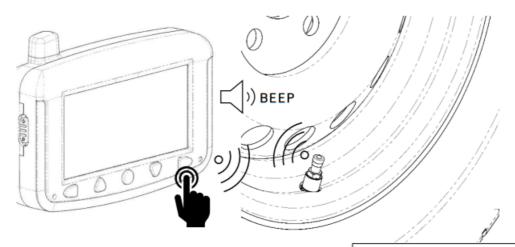
WITH THE MONITOR PREPPED AND THE DISPLAY SHOWING "FFF FFF" POSITION THE MONITOR WITHIN 50cm OR LESS OF THE SENSOR
