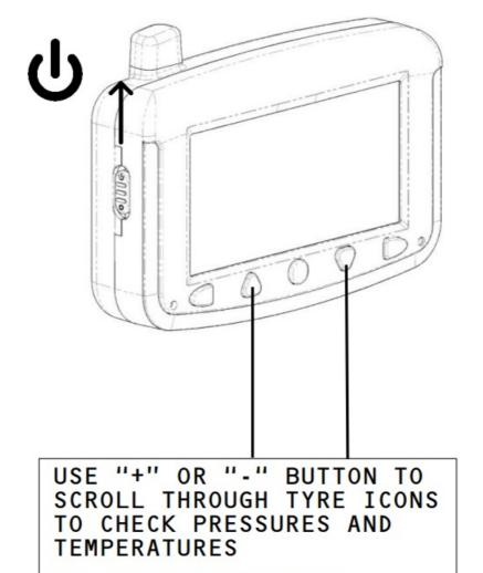
THE MONITOR DOES NOT NEED A PERMANENT POWER SUPPLY FROM THE VEHICLE TO FUNCTION. THE INTERNAL BATTERY PROVIDES APPROX. 60 HOURS OF CHARGE.
