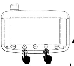
IF YOU WANT TO ADJUST THE FRONT AXLE HIGH PRESSURE ALARM PRESS THE + OR - BUTTONS TO RAISE OR LOWER IT. IF NOT KEEP QUICKLY PRESSING THE SET BUTTON FOR 1 SEC UNTIL THE AXLE YOU WANT IS FLASHING.
