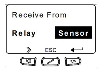
Now it's been configured to receive directly from the sensors you will now need to program the sensors into the monitor. Refer to next page. Before doing this, switch the monitor off and on using the switch on the right hand side of the monitor.
