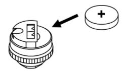
The Monitor will beep once the battery is inserted and the wheel location on the monitor will go solid black. Repeat this step for the rest of the new sensors until they are all programmed in and all-wheel icons are black. If the sensors do not program in keep removing and inserting the batteries until they do.
