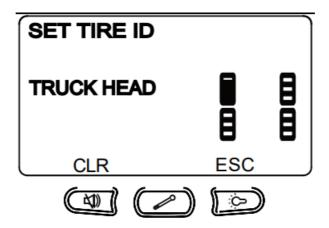
Now either switch the monitor OFF and ON using the switch on the side of the monitor. Or Press the Backlight (Right) button then the Temperature (Middle) button to exit the menu on the monitor. Test all sensors are working and programmed and set the Alarm Warning Thresholds if required.
