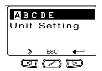
• Press the Mute (Left) button a couple of times to scroll across to menu C (Type of vehicle) then Press the Backlight (Right) button to enter this menu.
