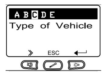
• TYPE of TRUCK HEAD and your current Layout No. will be displayed. Use the Mute (Left) or Temperature (Middle) button to scroll through the vehicle layouts to change if required and/or then press the Backlight (Right Button).
