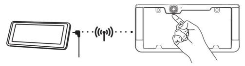
2. Plug-in 12V/24V power adapter to turn on the monitor. Turn on the camera by pressing the silver power button beneath the lens for 1 second. The blue LED status indicator will flash 2 times and an image should appear on the monitor.
