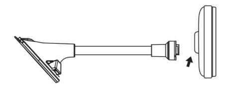
6. Mount and power the monitor. Power using the 12V/24V adapter provided. Remove overlay and adjust the angle as need.
