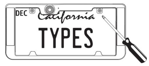
4. Align the camera with a license plate and secure it to the vehicle. See Manual for additional mounting guidance.
