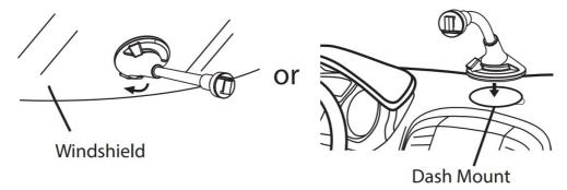
5. Place Windshield Mount on the windshield or Dash Mount and lower the lever to secure. Attach Dash Monitor onto the Windshield Mount and adjust to your desired position.
