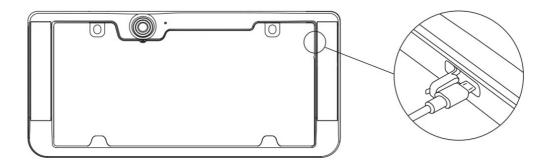
1. Fully charge the camera. Fold back camera power port plug and insert included charging cable. Most AC wall adapters will work with the USB charging cable.
