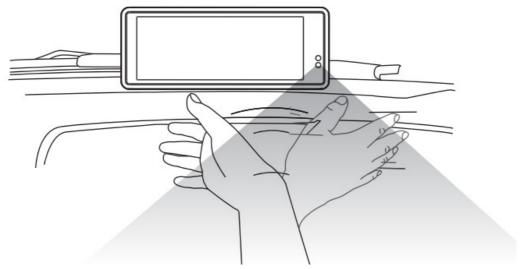
7. After the monitor has been connected to power, wake up the monitor and camera by waving your hand in front of the monitor, or tapping once on the screen.
