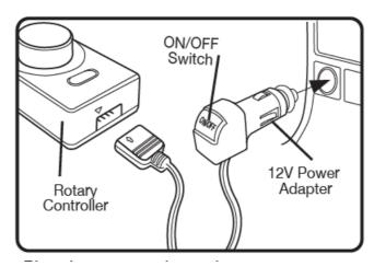
Plug the power adapter into a power socket and connect the other end to the Rotary Controller. Use the arrow indication to match the correct direction.
