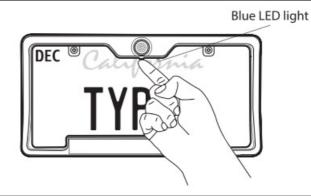
3. Push and hold the power button of the Quick-Connect Wireless Backup Cam for 1 second, the blue LED light will
