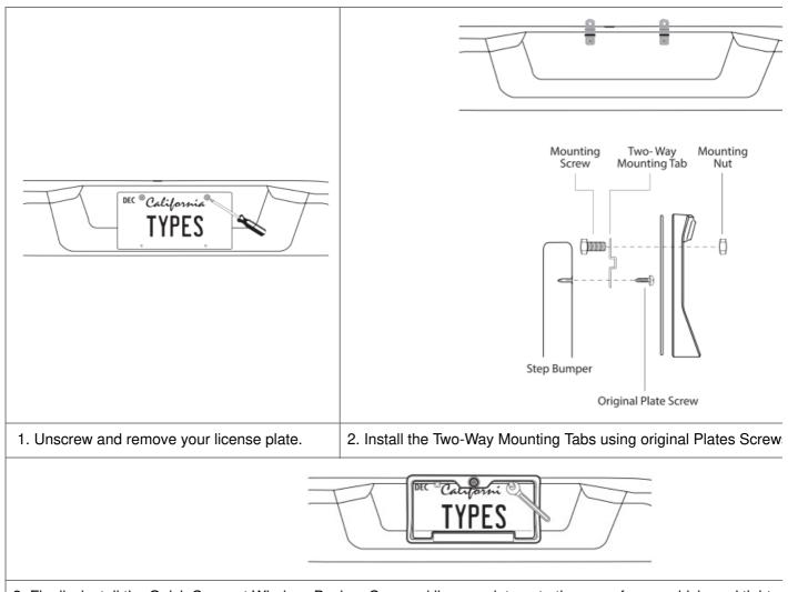
3. Finally, install the Quick-Connect Wireless Backup Cam and license plate onto the rear of your vehicle and tighter Mounting Nuts with a wrench.
