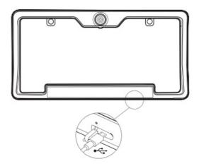
Open the camera power port plug cover and insert the charging cable. Most wall AC adapters will work with the USB charging cable .
