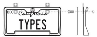
4. Secure the Quick-Connect Wireless Backup Cam with the license plate back onto the rear of your vehicle.
