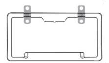
3. Install the license plate onto the Quick-Connect Wireless Backup Cam with the Mounting Screws & Nuts.
