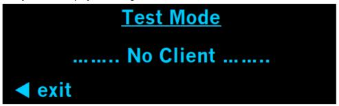
Get the client to lie on the bed/sit in the chair and the display should show "..... Client Detected....." Remain on the bed/chair for 10 seconds and the display will show "Unit is sending status IN code" After a short delay the display should show "..... Client Logged IN....."
