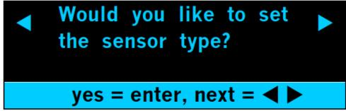
Press the ENTER key and the display will change to "Set Sensor Type; Bed Standard". Use the ▲▼ keys to select from; Bed Magic Stick or Chair Standard or Chair Magic Stick or Aux then press ENTER.
