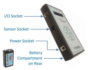
Plug the mains adapter into the Power socket and connect to the mains supply.
