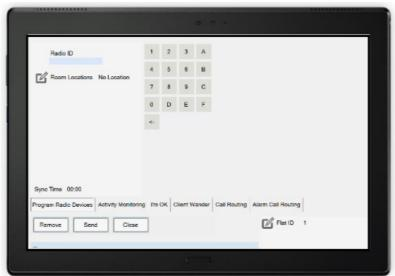
Press Flat ID and enter the flat number the sensor controller is being installed in. Enter 4-digits e.g. 0014.
