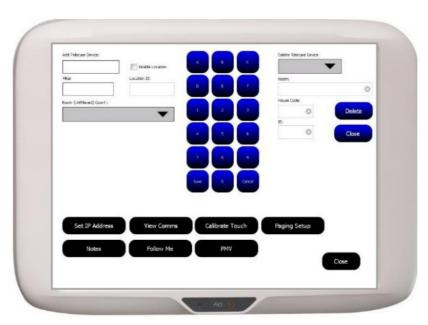
Touch the Add Telecare Device box and enter the Telecare device 10-digit Radio ID using the on-screen keypad. Touch the Filter box and enter the zone you want to add the Telecare device to using the on-screen keypad. Touch the Room box ▼ and select the Callpoint ID from the list that will be used to cancel the Telecare alarm. Touch the Save button on the keypad.
