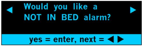
Press the ENTER key and the display will change to "Not in Bed Alarm; No"
