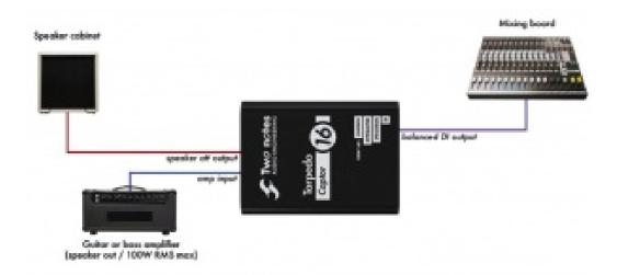
In this configuration, the amp is connected to the internal loadbox of the Captor. This means you have to match the impedance of the amp's speaker output and Captor.
