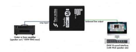
In the studio, it's best to use the dry signal of the amplifier and use the Wall of Sound plugin, for a more realistic speaker simulation. Plus, recording the dry signal means the virtual miking can be done and fine-tuned after the actual recording.
