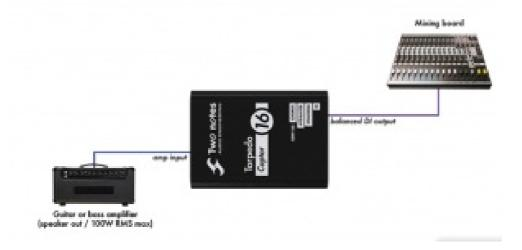
If silent miking is needed for a silent stage, you can remove the speaker cabinet of the previous configuration. Just connect the amp to the Torpedo Captor, and the DI output to the mixing console.
