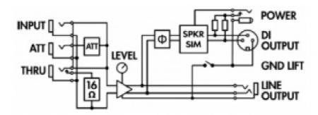
16 ohms version shows. The 4 and 8 ohms version have a 4 and 8 ohms loadbox, respectively, in place of the 16 ohms loadbox.
