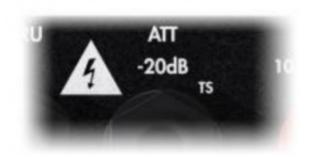
The ATT output provides a -20dB attenuation. Just plug a speaker cabinet in the ATT output (use a standard speaker cable for this connection), and crank up your amp while keeping a manageable volume.
