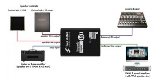
Please keep in mind that tube amplifiers MUST be connected to an appropriate load (cabinet or loadbox). Always plug the speaker output from your amp to the speaker input of the Torpedo Captor.
