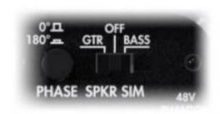
The speaker simulation embedded in the Captor is taken from our Le Preamp series. It's an analog simulation, featuring two models, Guitar and Bass, based on our Torpedo simulator. The Guitar model is based on our classic Brit VintC 4×12 picked up with a Dyn57. The Bass model is based on a mix of the vintage Fridge 8×10 and more modern Alu XL 4×10, picked up with a Cnd87.
