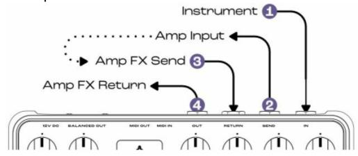
If your amp is equipped with an effects loop, add ReVolt's 3 channels to your amplifier's channel specification. Engage the 4-CABLE METHOD on ReVolt, and combine ReVolt's effects loop with the amp's using the following connectivity guidelines.
