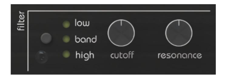
The SID chips are equipped with a multimode resonant filter.
