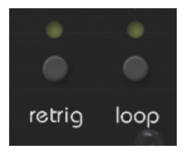
the LFOs can be used as "one-shot" envelopes by deactivating the looping feature using the loop button. This is useful for achieving pitch decay on percussive sounds and other effects. Additionally, the LFOs can be retriggered on every key press by toggling the retrig button.
