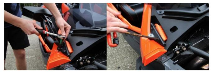
4. Starting from the rear, place the frame on the Slingshot. The two back plates go on the back headrest on the front of the roll hoop. Attach and tighten halfway with four shorter/skinnier bolts (35mm). The four long bolts (12mm) go into where the mirror brackets were. Tighten halfway on each side. Once all bolts are in place, tighten the remaining bolts. Put mirrors back on with same OEM bolts.
