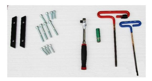
1. After unwrapping, put the two-piece frame together with bolts provided. (3/8 shorter/fatter bolt)
