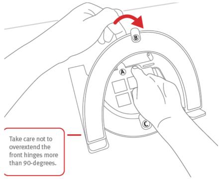
3. Hold down the back hinges while carefully lifting Curve Flex until you feel it stop.
