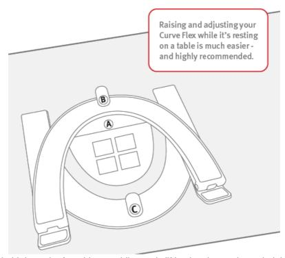
2. To raise Curve Flex, hold down the front hinges while gently lifting it to its maximum height. Take care not to
