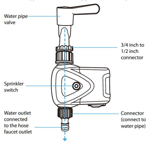
3. After installation, open the water pipe valve and pair the equipment distribution network to the APP according to the instructions to use it
