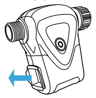
3. Install 4xAA battery, Replace the battery compartment.
