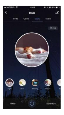
• The 1-4 scene is static color for all light type. the inner color of this scene can be editable. The 5-8 scene is dynamic mode for RGB type, such as green fade in and fade out, RGB jump, 6 color jump, 6 color smooth.
