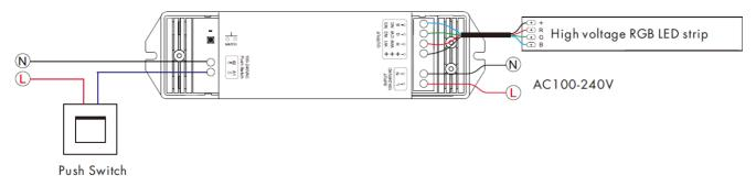
Press and hold the match/set key for 12s, until the RUN LED indicator turn red, then release, the controller will become RGB type, then do smart con?g by tuya APP, or short press match key to match with RGB RF remote.
