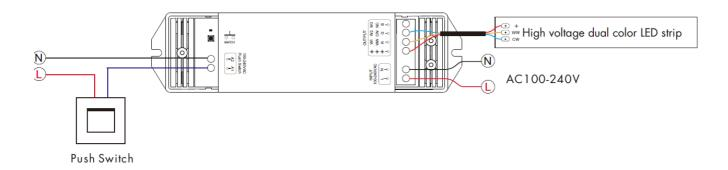
Press and hold the match/set key for 10s, until the RUN LED indicator turn yellow, then release, the controller will become CCT type, then do smart con?g by tuya APP, or short press match key to match with CCT RF remote.
