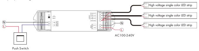
Press and hold match/set key for 8s, until the RUN LED indicator turn white, then release, the controller will become DIM type, then do smart con?g by tuya APP, or short press match key to match with dimming RF remote.
