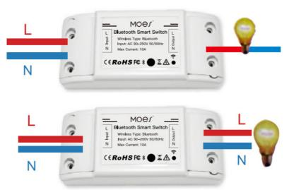
Note: The Bluetooth Switch must be powered up by N and L wires.
