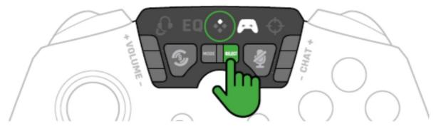
3. Activate Mapping Mode by holding the SELECT button down for 2 seconds. The profile lights will blink.
