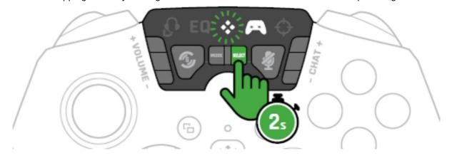
4. On the bottom of the controller, press the Quick Action button you'd like to map to.
