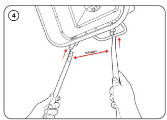
Thread the M6x35 bolt (12) through the hole of the handle bar (item 2) and lower frame (item 15). Use the M6 wingnut (13) to tighten. Repeat on both sides.
