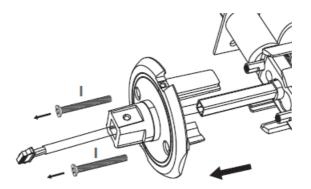
• Remove the latch assembly. It is now ready for installation.
