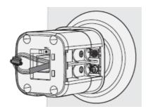
• Install 4x AAA batteries into battery compartment. Cover the inside knob over battery compartment and make sure the side with inside screw is downward. Use the hex key to tighten the inside screw (clockwise) to complete the installation.
