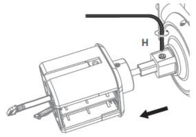
• Loosen the inside screw (counterclockwise) on the bottom of the back plate cover and remove it.
