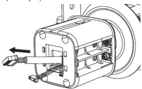
• Loosen the inside screw (counterclockwise) and gently remove battery compartment without pulling or breaking the power cable.
