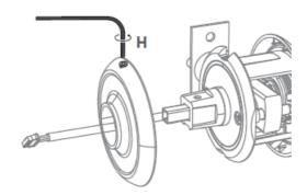
• Unscrew the back plate and remove it. Do not pull on the power cable.
