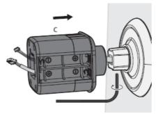
• Gently pull out the power cable connectors and snap them together. Once connected, gently collect the two cables back into the battery compartment.
