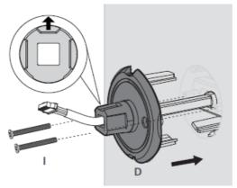
• Feed the power cable through the back plate cover, and cover it on the back plate part, then use the hex key to tighten the inside screw (clockwise) at the bottom of back plate cover.
