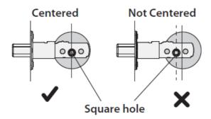
• Latch Adjustment (only if needed): Hold the front of the latch and the square opening from both sides, pull or push to extend or retract the latch end as needed.
