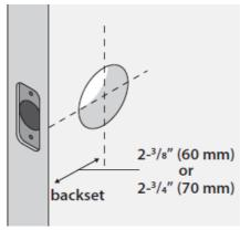
• Make sure that the hole in the door edge is 1" (25 mm).
