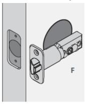
• If the square hole in the latch is centered in the door hole, no adjustment is required. If the square hole is NOT centered, adjust latch. See "Latch Adjustment" (step 3C)
