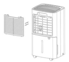
• **b)** Use a vacuum cleaner to gently absorb the dust on the surface of the filter. If the filter is very dirty, wash it with water and a soft detergent and dry it thoroughly afterwards.
