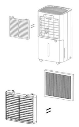
3. Mount the T-CLEAN filter with the frame on the unit
