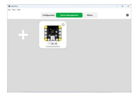
Click on the expansion symbol in the upper right corner of the device. If you have connected multiple devices, click on Recognize, and the status indicator of the selected device will flash green; if you need to disconnect from the selected device, click on Disconnect.
