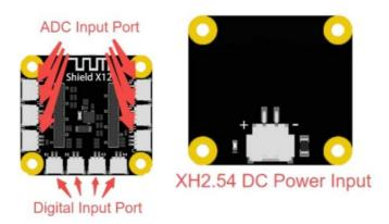
On the left and right sides of the transmitter shield, there are 3 ADC input channels respectively. Below it, there are 4 digital input channels. The gray slot on the back is the slot for the multi-function controller core. It can be powered through the XH2.54 power input.
