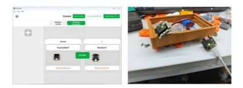
After modifying the configuration, remember to save the configuration locally with Save Config in the upper right corner, and update the configuration to the device with Send Config.
