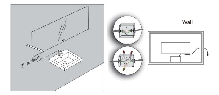
Use the tape measure the height, and draw the horizontal, line and the vertical line of the wash-basin. Measure the distance of the mirror hole, and mark the hole place on the wall.
