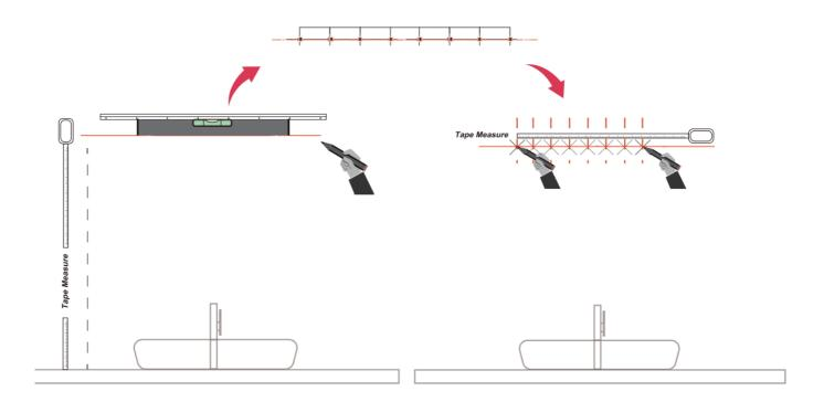
Drill and insert the Wall Anchor, Drive in the screw cross the bottom support.
