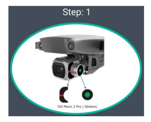
Mount the green tracking mark sticker aligned to the circle on the aircraft's camera. Mount the red tracking sticker on the aircraft's camera (see illustration).
