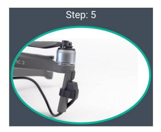
Slide the cable plug upwards until it reaches the front LED. Slide it upwards until it fully covers the aircraft's front LED. Fasten the cable below the drone's arm with the Velcro.
