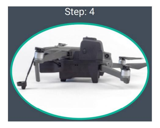
Make sure the battery is mounted securely and that the battery latches have clicked into place. The image illustrates a correctly mounted battery. There should be no «GAP» between the battery and the battery connector on the Automating light unit.
