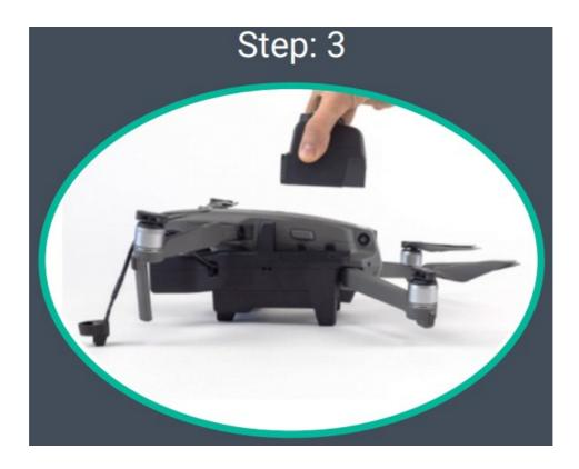
Insert the Autoboxing light Battery into the Automating light's battery slots. Slide the battery forwards to the Automating light's battery compartment.
