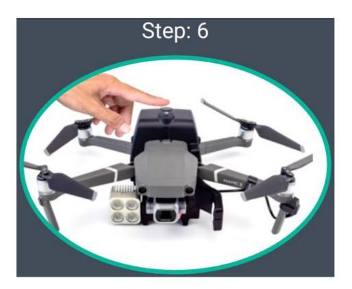
Hold the power button on the battery down for around 3 seconds to turn on the Automating light. On startup the floodlight LED will blink once, when the boot sequence is ready the lamp will blink one more time.
