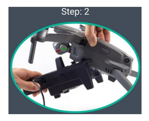
Slide the Automating light unit above the belly of the aircraft above the rear aircraft arm while maintaining a 45° angle. As you do this, begin to adjust the Autoboxing light unit's angle so that, after the end of the sliding motion, it is parallel to the aircraft's body.
