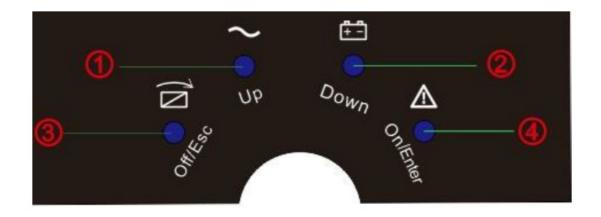
① Inverter LED ② Battery LED ③Bypass LED ④Alarm LED
