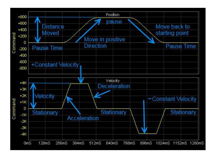
The parameters used to generate the above waveforms are shown here. Note the "Distance" moved of 800 steps, the "Velocity" of 4000 steps/sec and the "Pause Time" of 250ms. The Wave Generator parameters are located on the "Tuning" tab.
