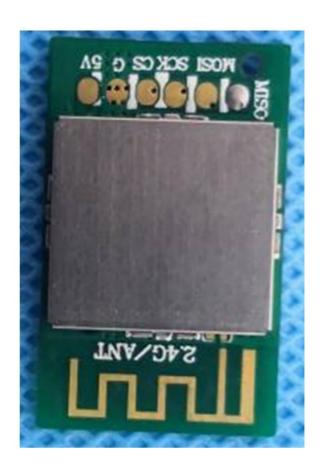
Based on the Bluetooth BLE 5.3 SOC scheme Small size: 27x14x1mm
