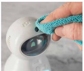
• When cleaning Kitt, please ensure that its teal cleaning cap is securely attached to prevent water damage to the charging port and switches.
