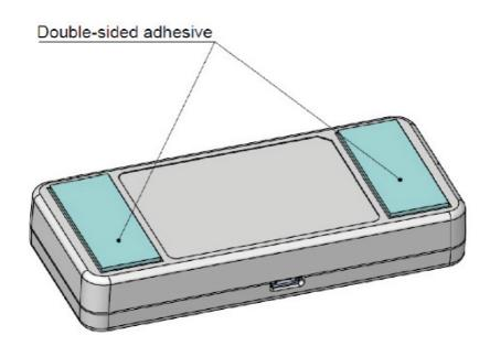
If the device is mounted on metallic surface, or close to substantial amount of metal the antenna performances may be compromised. To achieve full function antenna performance the device should be mounted no less than 30 mm from metal. Avoid placing the device close to powerful electromagnetic equipment.
