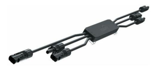
The TSOL-RSDM-DD/DS/CQ is a rapid shutdown device designed to be fixed on the frame of solar modules or on the wall. It is part of the rapid shutdown control system that can control up to four strings of solar modules. The device has input and output connectors for DC cables and an AC cable port for connecting to a power source. The rapid shutdown controller is used to turn on or off the rapid shutdown devices in each string of solar modules.
