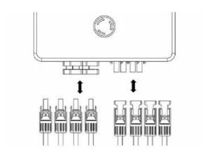
• Each rapid shutdown controller can control four strings of solar modules.
