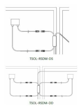
• Then connect the outputs of all the rapid shutdown devices one after another.
