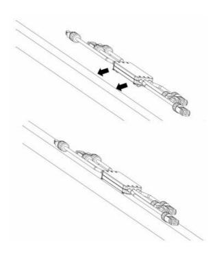
Step 2: Connect the rapid shutdown device
