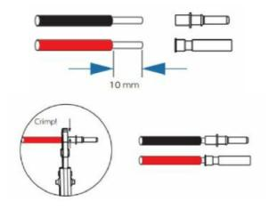
Tips: Use AWG 12 (or 4 mm2) cable for DC cable.
