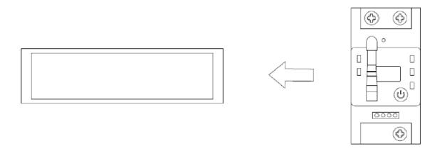
**Step 3:** Connect the L (live wire) line of the three – phase switch to the L  $\downarrow$  port of the Smart Meter, where L  $\downarrow$  is the input port, from the power grid to the meter. Connect the L (live wire) line of the single – phase switch to the L  $\uparrow$  port of the Smart Meter, where L  $\uparrow$  is the output port, from the meter to the household load. Connect the N (neutral wire) line to the N port of the Smart Meter.
