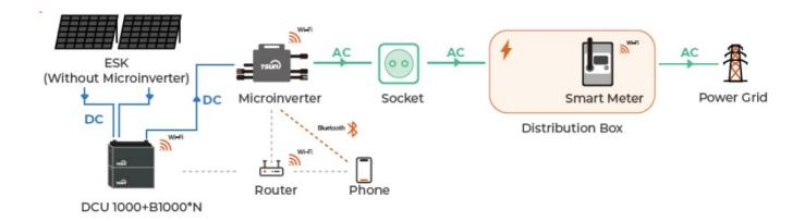
**Example 2:** Smart Meter and Microinverter Systems
