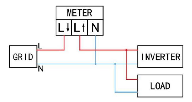
**Step 4:** After confirming that the wiring of the meter is correct, turn on the three-phase switch and the single-phase switch.
