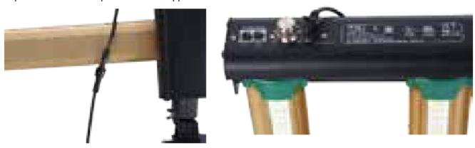
• After both bars have been installed connect them on to each other and finally plug in the power cord into the ROI-E720 12v plug.
