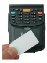
Correct orientation; the transponder is parallel to the reader antenna and read range will be good.
