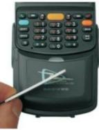
Incorrect orientation; the transponder is perpendicular to the reader antenna and read range will be poor.
