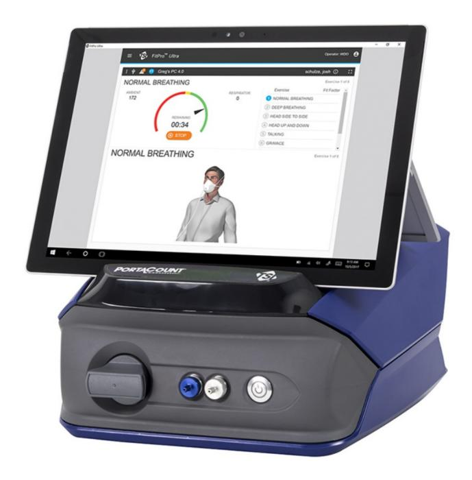
FitPro™ Ultra Fit Test Software is capable of conducting both quantitative and qualitative fit tests. This guide describes the operation and menus of the Qualitative Respirator Fit Testing option.
