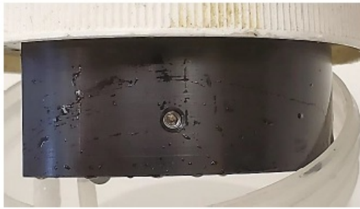
Figure 5 Location of the Dilution Air Set Screw
