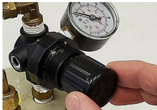
Figure 4 Adjusting the Pressure Regulator
