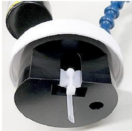
Figure 3 Atomizer Liquid Draw Tube
