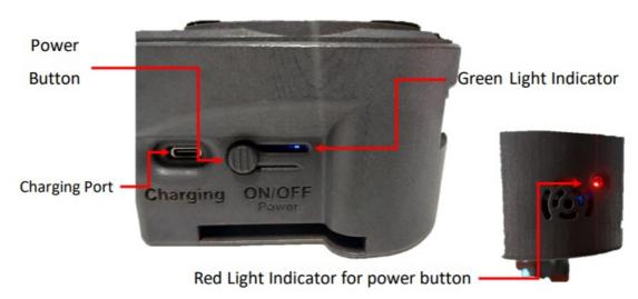
• While charging, the indicator will show a blinking green light. The number of green bars (Maximum of 4) indicate battery charge level.
