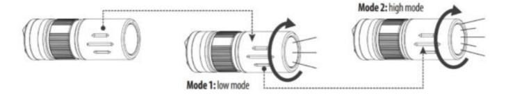
**ON/OFF:** output changes are controlled by twisting the flashlight head. Twist slightly to turn it on at 5 lumens and a bit further for 220 lumens.
